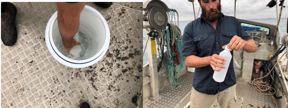
5. Leave a small airspace at the top of the sample bottle and ensure the cap is screwed on (see picture above).
