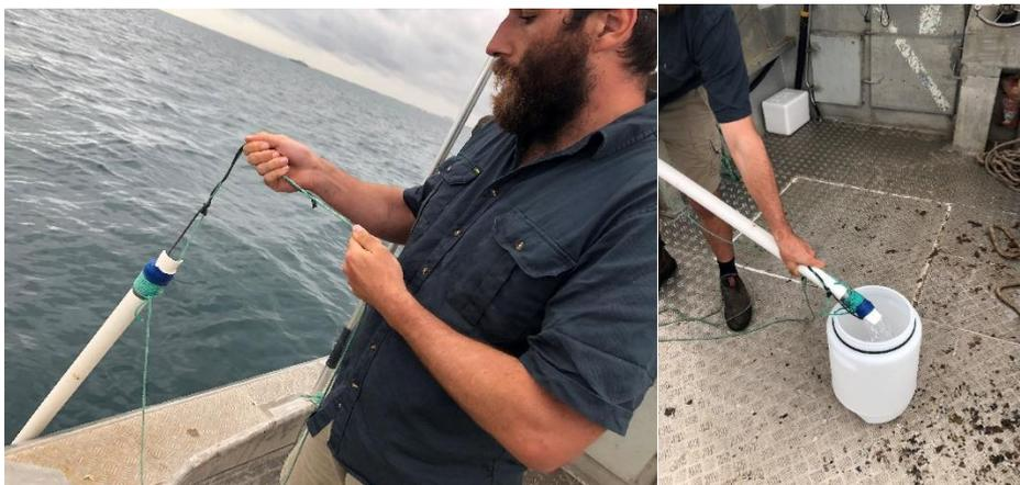
4. At those sites where the water depth is less than 2m and the water column is well mixed, a bucket with a rope attached should be used to collect the water sample. Avoid stirring up the sediment before sample collection. Collect at high or incoming tide. Mix the contents of the bucket and immediately fill the sample bottle to the neck by immersing the bottle in the bucket (see picture below). Do not allow the contents of the bucket to settle before filling the bottle.
