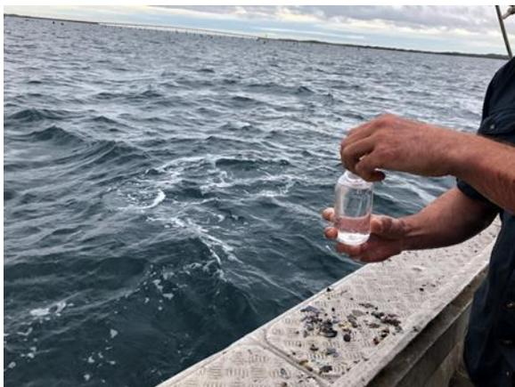
8. Carefully replace the screw-cap immediately and tightly.
