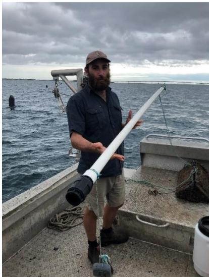
2. Remove the bung from the bottom end of the tube/pipe sampler. If using one-way foot valve as pictured, open the valve using the rope. Lower the weighted end valve end carefully using the rope (so as not to disturb any layers of phytoplankton in the water column). The pipe must remain vertical in order to take an even sample of the whole water column.
