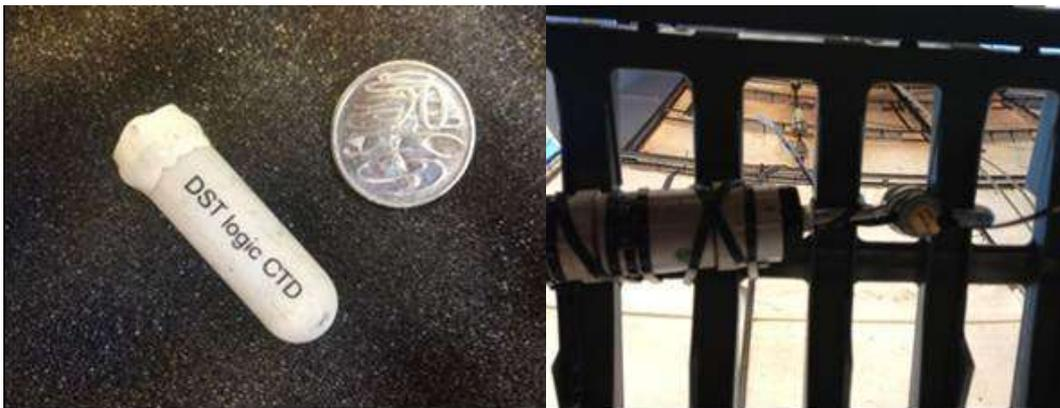
**Figure 8.10.** Image of the conductivity, temperature and depth logger used to assess the environmental condition.
