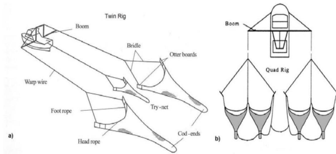
**Figure 2.2. Standard (a) twin-rig and (b) quad-rig otter trawl (Adapted from Stirling 1998). The quad-rig configuration is currently used by all vessels in the SBPMF.**
