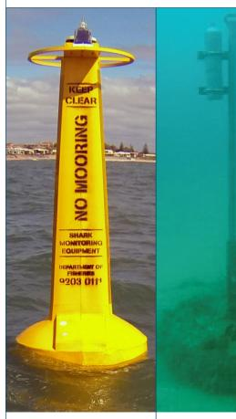
Satellite-linked (VR4G) acoustic receivers transmit detection data in real-time via satellite.
