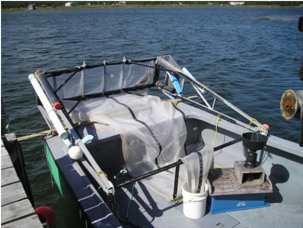
Figure 2. Net in “pull” configuration setting on the stern of a 10 m lobster fishing boat. Note the plastic pipes attached to the left side of the frame for flotation, the reflector plate at the right rear of the frame, and the spreader bar between the arms.
