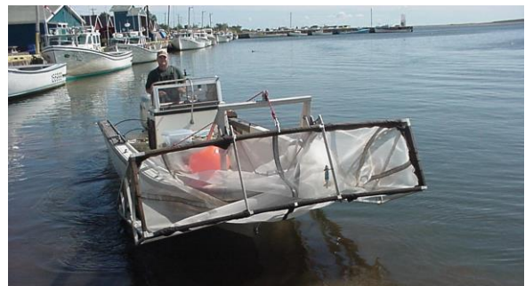
Figure 1. Net in "push" configuration resting on the bow A-frame.
