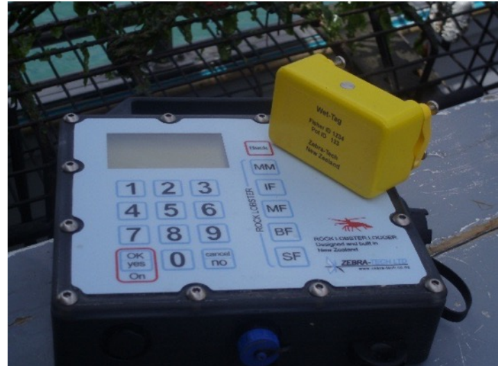
Deck Logger and Wet-Tag, low cost and easy to use technology for fishermen
