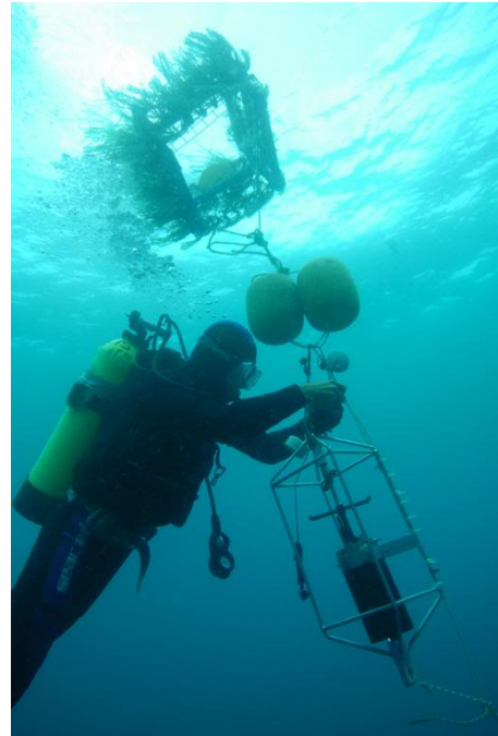
Figure 2. SCUBA diver attaching current meter to one design of a passive post-larval collector for Jasus frontalis . (Photo credit: R. Wahle).
