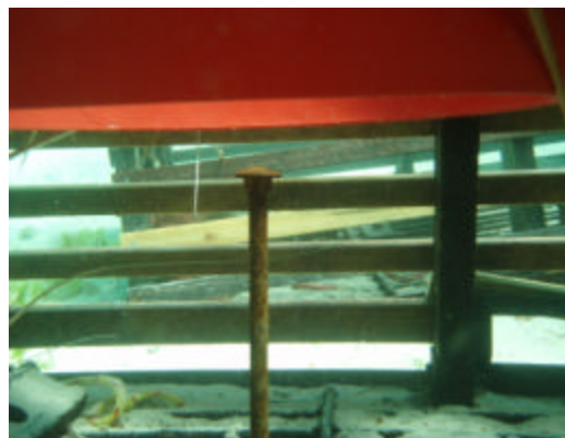
Figure 2b. SLED consisting of an upright attached to the bottom of the pot and finishing near the bottom of the neck.
