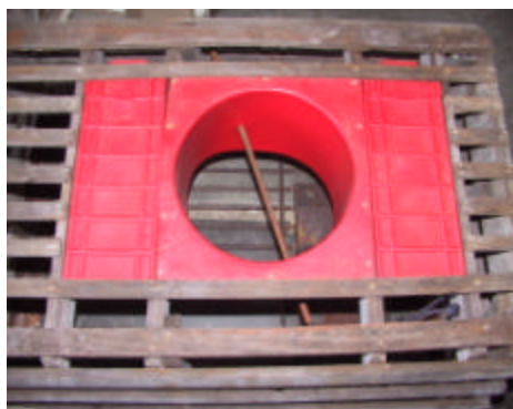
Figure 2a. SLED design consisting of a straight metal bar through the neck of the pot.
