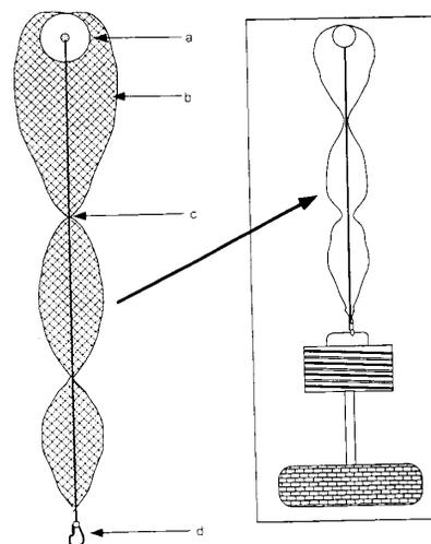
Figure. Mesh collector (left) and modified crevice collector (right). The mesh collector consists of a) 15 cm diameter styrene float; b) nylon trawl mesh bundled and tied to the main float line; c) 8 mm rope connecting snap clip and float; d) snap clip for attaching mesh to the top of a standard crevice collector.
