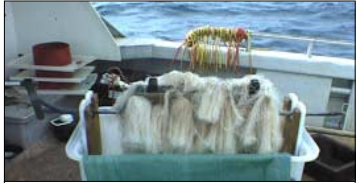
Figure 4: Spinning tub for sampling collectors.
