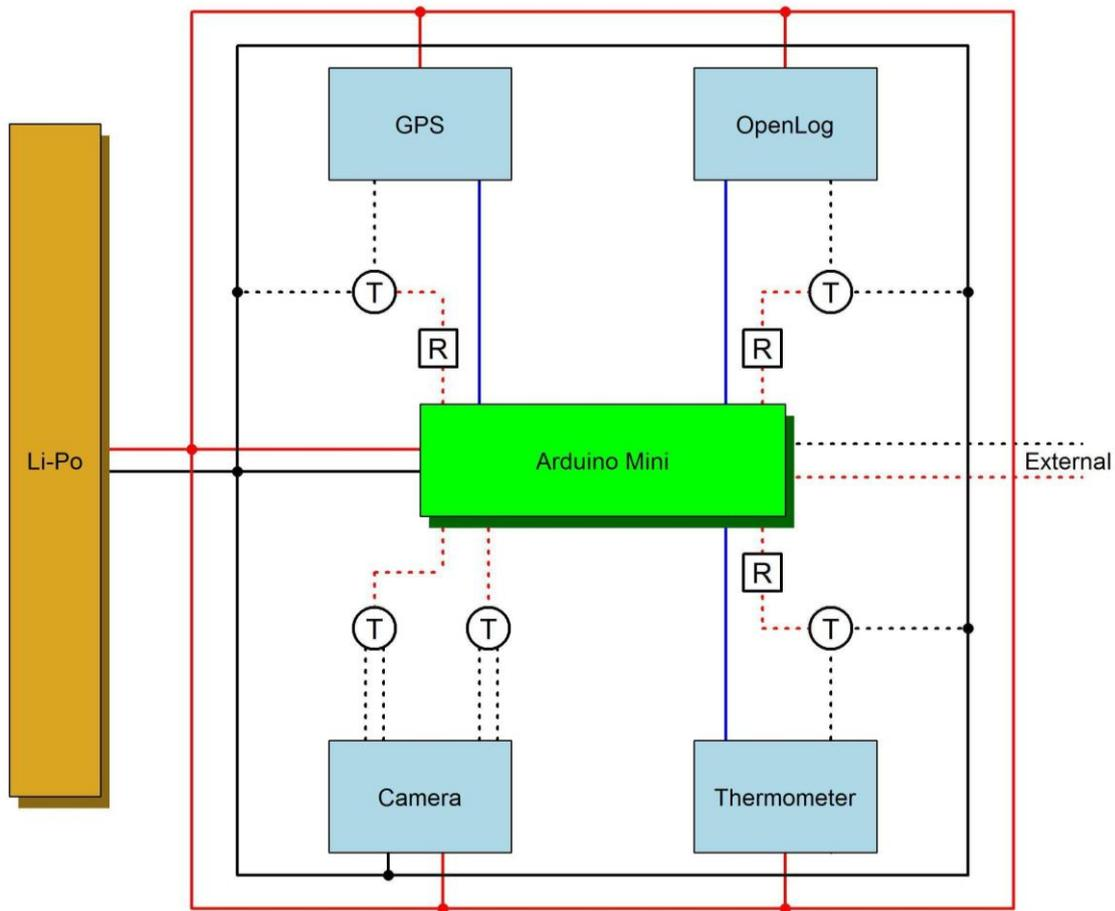
**Figure 2.** Wiring schematic of the POTBot, with permanent connections shown as solid lines and intermittent connections as dotted lines. Red, black and blue lines denote positive, negative and serial (data) connections, respectively. Transistors (T) and resistors (R) are shown. The external wires shown at the middle right are the wires running to the external of the water housing to detect the presence of water.
