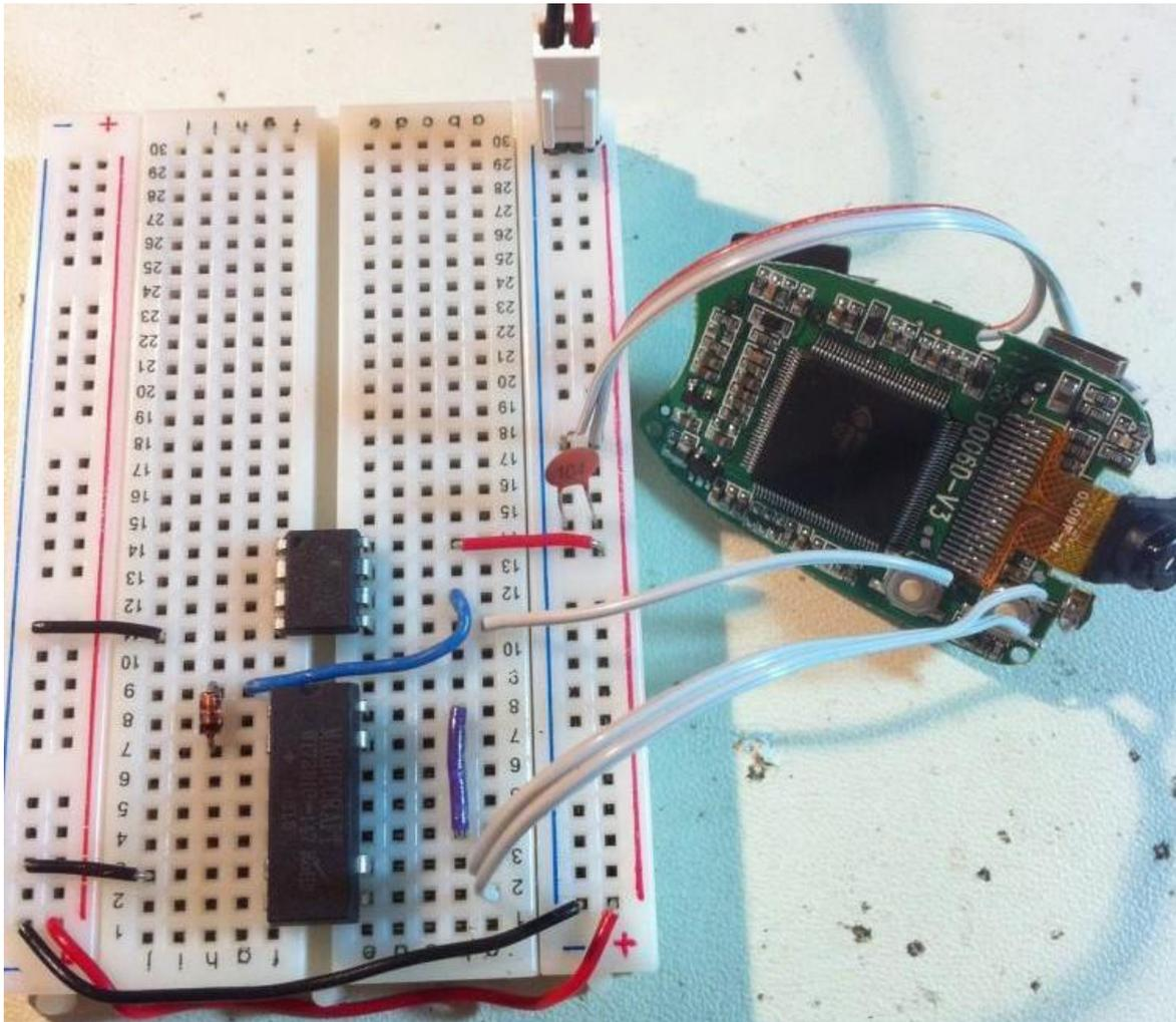
**Plate 1.** Breadboard linking power to an integrated circuit and an 808 camera, using a signal relay to connect a junction across the shutter button on the camera (paired white wires) (photo from <http://quinndunki.com/blondihacks/?p=925>).
