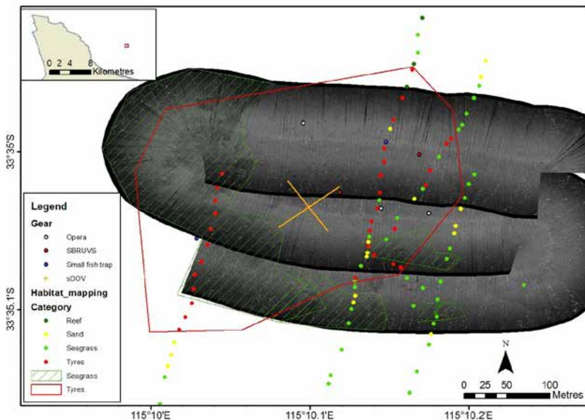
**Figure 7.12** Sidescan sonar map of Quindalup tyre artificial reef site showing sampling locations, towed video benthic habitat observations and indicating areas of seagrass (green hatching) and area with tyres (red).
