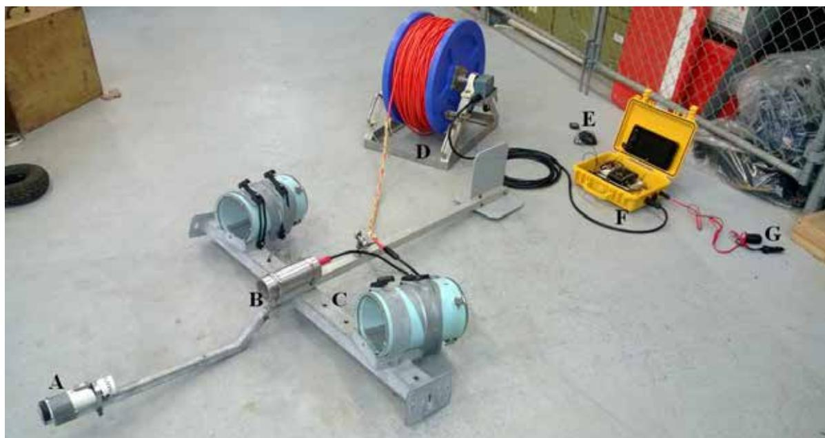
**Figure 2.2** Towed underwater video setup utilised on the smaller research boat where A- synchronising diode, B- live feed video camera, C- BRUV crossbar with stereo video housings, D- live feed video cable, E- GPS overlay antennae, F- topside case with monitor, video out plug and GPS overlay and G- 12v power supply .
