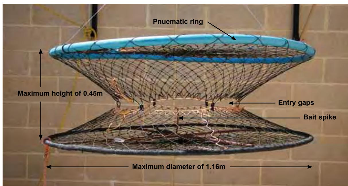
**Figure 1.2.** Hourglass trap used by commercial blue swimmer crab fishers in Cockburn Sound.
