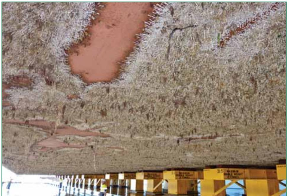
A heavily ‘biofouled’ commercial vessel hull.
