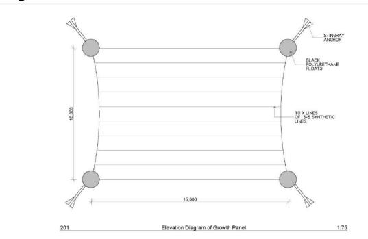
Figure 1: Production Panel configuration
