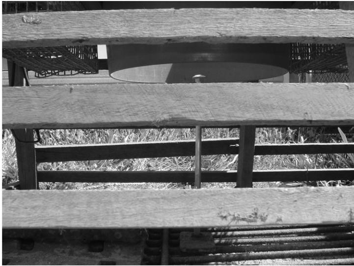
**Figure 6.** The modified SLED to be trialed in the 2004/05 WRL season. This device consists of a galvanised cup-head bolt that screws into a fitting welded to the bottom of the pot.
