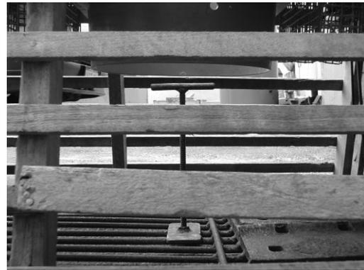
**Figure 4b:** T-bar exclusion device (220mm high X 100mm wide) and the welded female fitting on the base of the pot.
