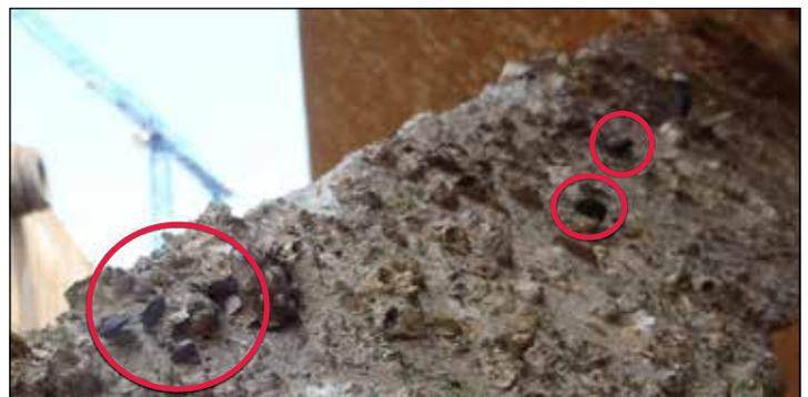
Asian green mussels on a vessel's zinc anode demonstrating how difficult they can be to detect. Photo: John A. Lewis
