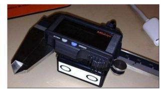
Figure 8.8. Digital Vernier callipers with Bluetooth box for wireless transfer to the iPhone, which is activated when one of the two buttons for male and female is pressed
