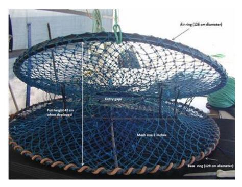
Figure 4.2. Example of a collapsible crab trap permitted for use in the SBCMF. Non-collapsible traps are also used.
