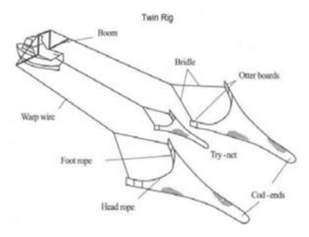
Figure 2.2. Standard twin-rig otter trawl (Adapted from Stirling 1998) that is currently used by all scallop vessels in the AIMWTMF.
