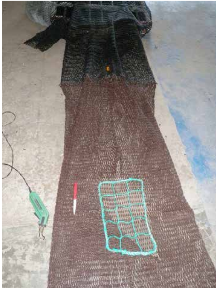
Figure 9.2. Austral grid equipped with an appropriate sized Dynex netting extension and codend (i.e. 150 meshes around)
