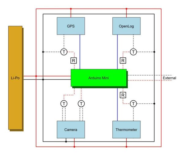
**Figure 2.** Wiring schematic of the POTBot, with permanent connections shown as solid lines and intermittent connections as dotted lines. Red, black and blue lines denote positive, negative and serial (data) connections, respectively. Transistors (T) and resistors (R) are shown. The external wires shown at the middle right are the wires running to the external of the water housing to detect the presence of water.
