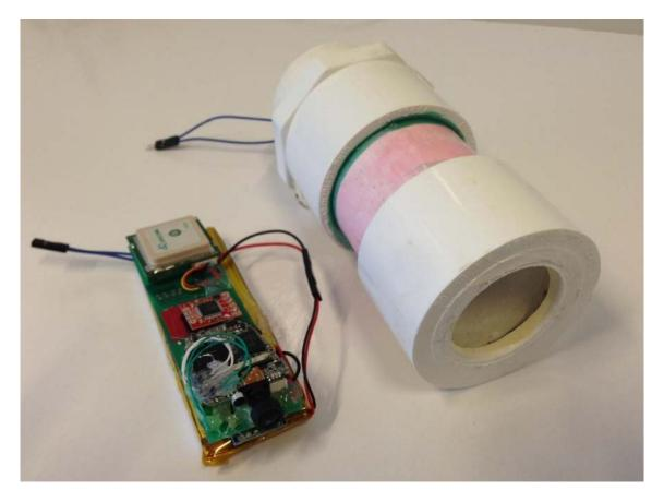
**Plate 4.** POTBot built on purpose-made PCB (green) with camera at the front, GPS visible towards the back and battery and Arduino mini located under the PCB; PVC underwater housing capable of deployments down to 180 m depth.
