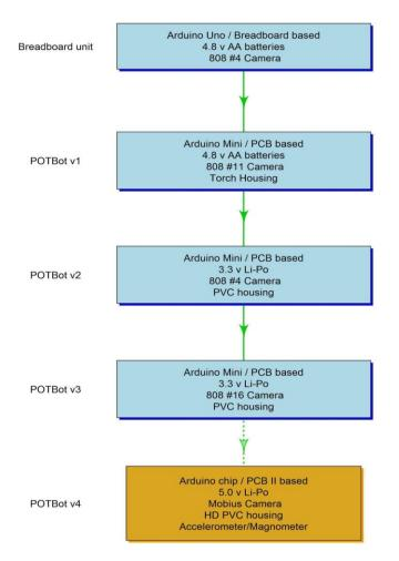
**Figure 1.** Evolution of the various versions of the POTBot. Note version 4 was developed subsequent to the analyses described in this report.
