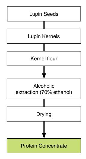
Figure 13.1 Schematic flow chart for the production of lupin concentrate.
