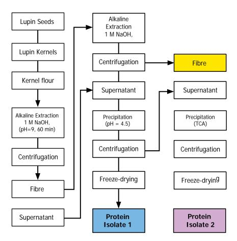
Figure 13.5 Flow diagram for the production of Lupin Fibre, Protein Isolate 1 and Protein Isolate 2.
