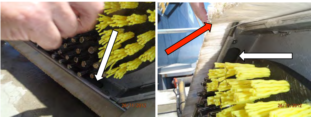
Figure 2.2 Under surface of cart showing suction ports (white arrows) and shroud (red arrow).
