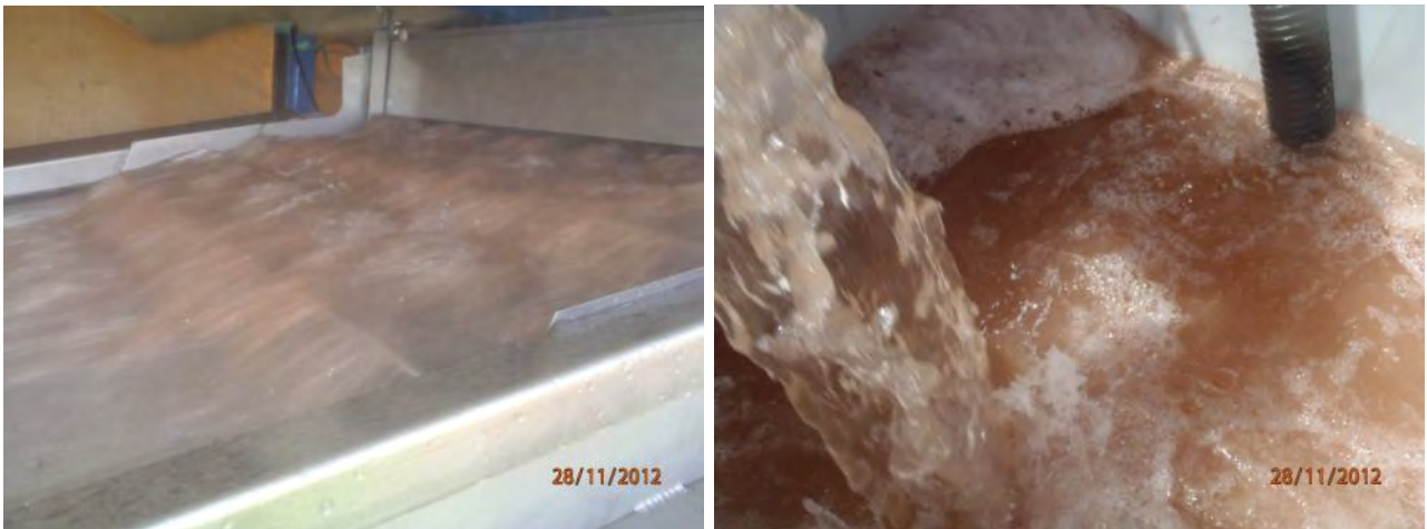
Figure 6.7 Red (copper) tinted water flowing over the first stage filter (left), filtrate in the tank below the filter tray (right), during the Wambiri hull clean.
