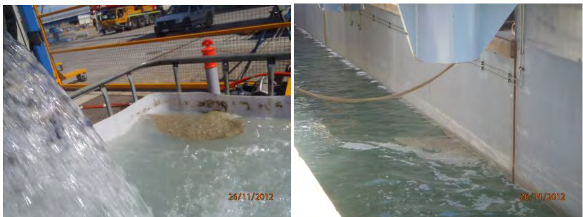
Figure 4.6 Organic scum derived from the filtrate in the discharge tank (left) and beside the Yargan (right).
