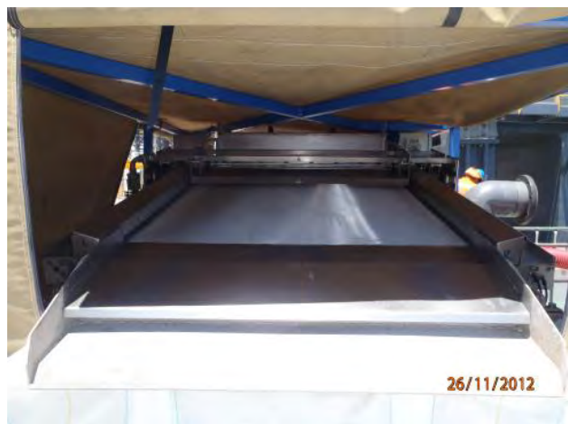
Figure 2.6 First stage filtration: filter screen
