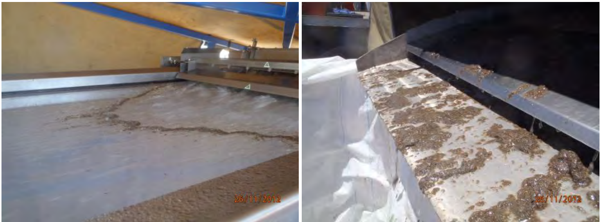
Figure 4.4 Debris greater than 50 \mu\text{m} accumulating on the baleen screen (left) and washed into the waste bag (right).
