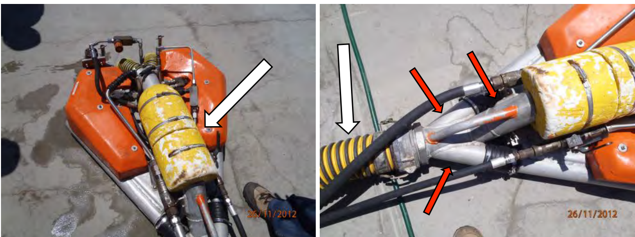
Figure 2.3 Upper surface of cart showing, left, buoyancy float and, right, suction outlets (red arrows) and hose (white arrow).
