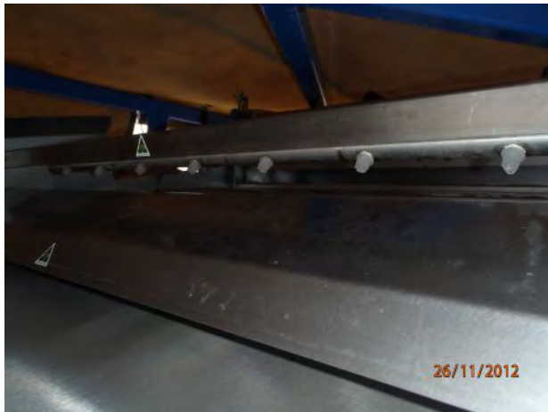
Figure 2.7 First stage filtration: upper and lower spray bars
