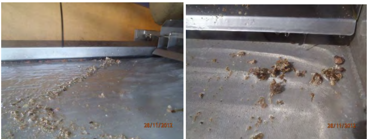
Figure 6.8 First stage filtration debris from the box clean of the Wambiri anode (left), and scraper clean of the jetty pile (right).
