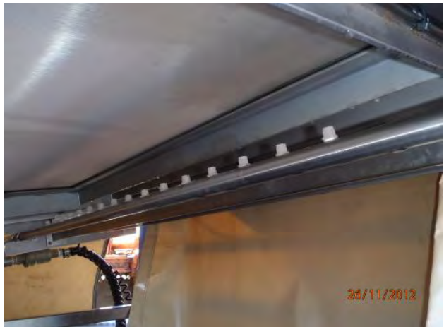
Figure 2.7 First stage filtration: upper and lower spray bars
