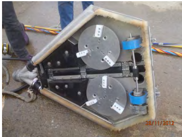
Figure 2.4 Cleaning heads with non-contact nylon blades.
