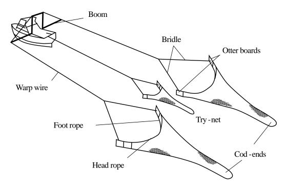
Figure 5. The standard twin otter rig and try gear used by prawn trawlers in Shark Bay.
