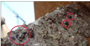
Asian green mussels on a vessel's zinc anode demonstrating how difficult they can be to detect. Photo: John A. Lewis
