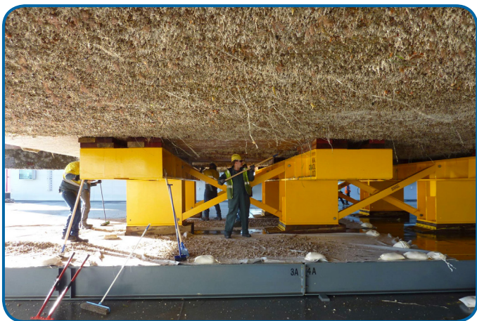
Heavily biofouled vessel being cleaned in dry dock to reduce risk of invasive species translocation
