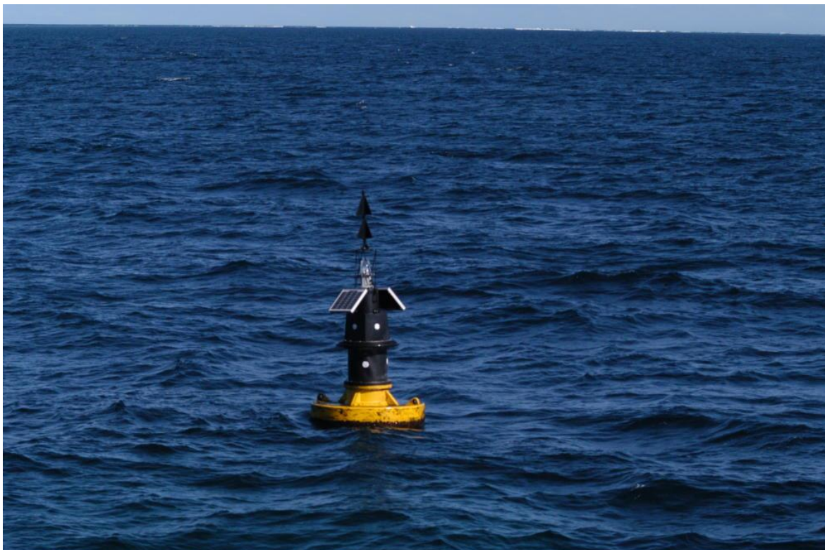
Image 34- solar powered north cardinal marker navigation aid, Middle Island Pelsaert Group. Credit: DPIRD.
