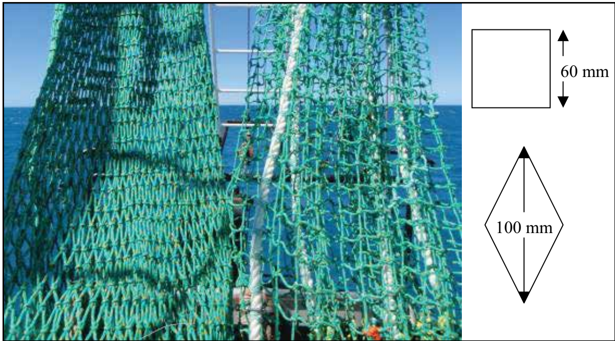
Figure 3.2. Examples of meshes trialled; standard 100mm (stretched length) diamond mesh codend used by the scallop fleet (left) and the 60 mm (knot to knot) square mesh codend (right). Mesh sizes refer to the distance between corner knots on the square mesh codend net and the stretched measurement from knot to knot on the diamond mesh codend net.
