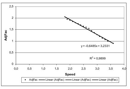
**Figure 3.8** Adjustment factor in relation to trawl efficiency with speed compared to a standard 3.4 knot.
