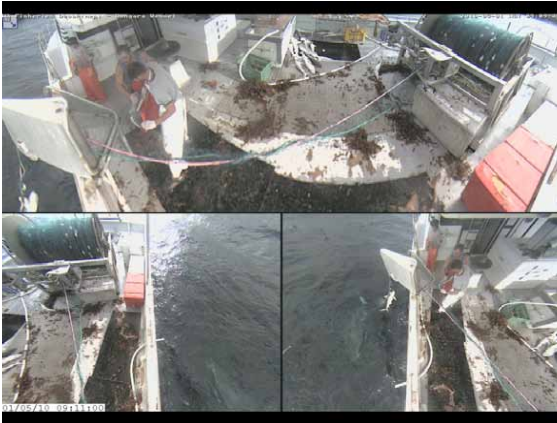
Figure 2. Examples of views from the 360° Mobotix Q24 camera. Top image shows the deck and gillnet being hauled onto the roller. Bottom left is the view to the stern from the camera position and the bottom right is the view forward of the camera observing the net coming out of the water with the catch. In these images note the catch in the top screen, fishers removing a shark from the net, while two more sharks are pulled up to the surface (lower images).
