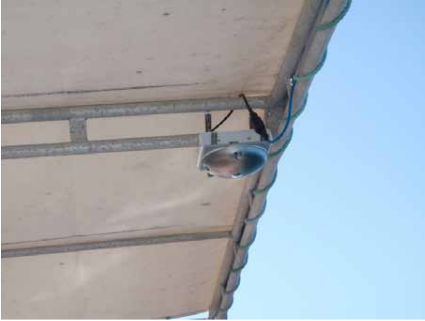
Figure 1. A Mobotix Q24 camera mounted on a commercial gillnet vessel in Dongara to monitor catch, bycatch and protected species interactions.
