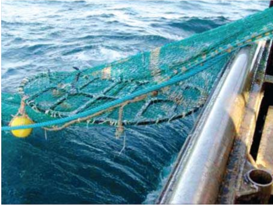
Figure 2. “Evaflex” grid being hauled aboard a French sea-bass trawler.
