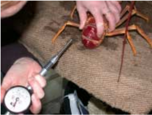
Figure 1: Using a durometer to test the shell hardness of the abdomen of a male southern rock lobster, Jasus edwardsii .
