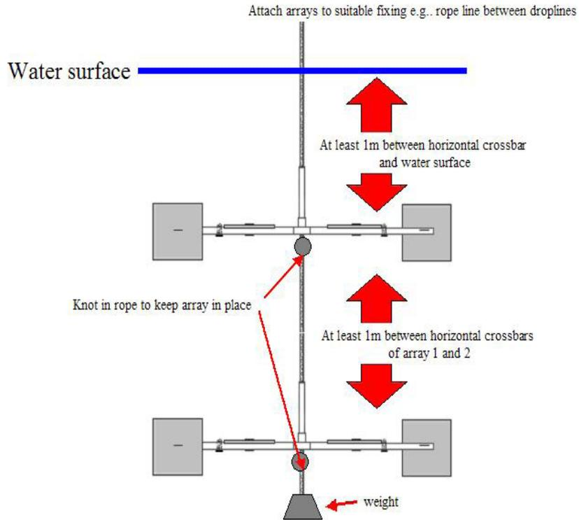
**Figure 13.** Schematic of the settlement plate system showing two arrays connected via a single rope line. This free hanging assemblage requires a weight at the bottom.
