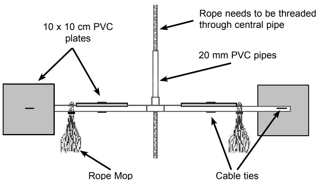
**Figure 12.** Illustration of the settlement plate arrays showing one vertical and one horizontal plate attached to each of the two arms of the system. Adapted from Marshall and Cribb (2004).
