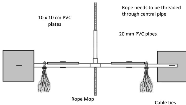
**Figure 1: Illustration of the settlement plate system showing one vertical and one horizontal plate attached to each of the two arms of the system. Adapted from Marshall and Cribb (2004).**
