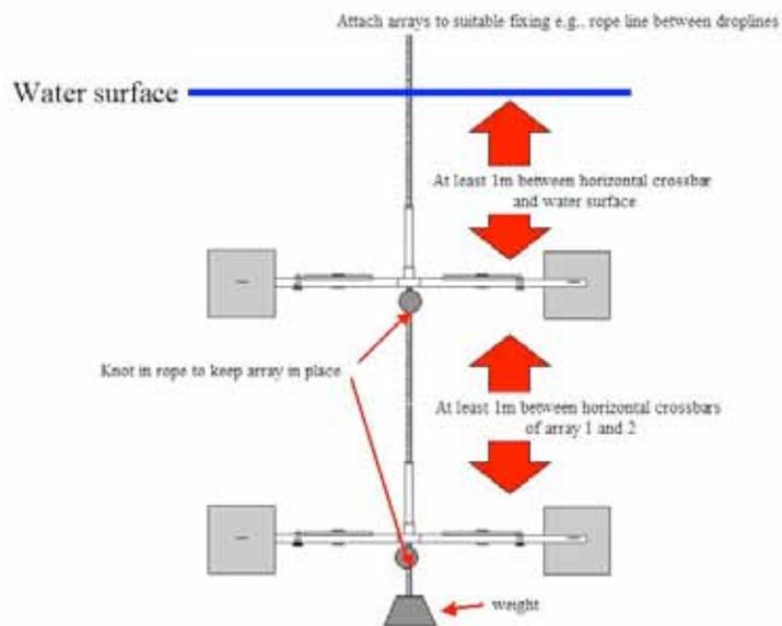
Figure 2: Schematic of the settlement plate system showing two arrays connected via a single rope line. This free hanging assemblage requires a weight at the bottom.
