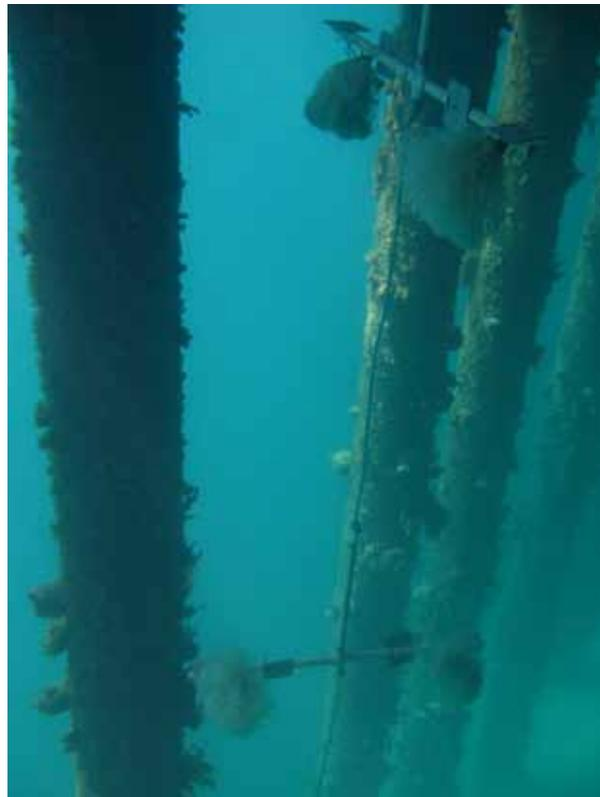
**Figure 14.** Arrays *in-situ* – showing rope collectors and multiple arrays connected by rope to sample at different depths.
