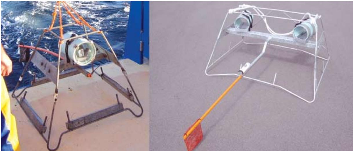
**Figure 2.14.** Single (left) and stereo (right) camera systems used in the project.
