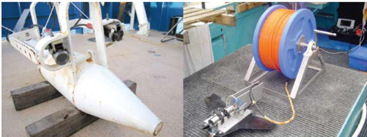
**Figure 2.16.** Towed camera setups used in the current project. Left; dual camera live-feed system used onboard the *RV Naturaliste*. Right; single camera paravane system used onboard the *RV Snipe*.
