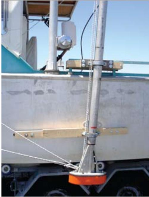
**Figure 2.7.** Simrad EQ60 mounted on board the RV Snipe.
