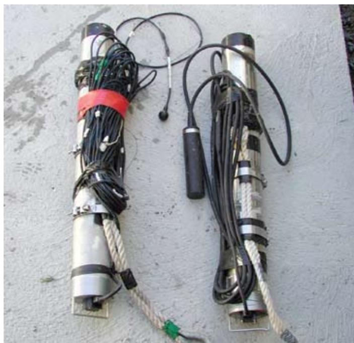
**Figure 2.12.** Acoustic logger housing with hydrophone.
