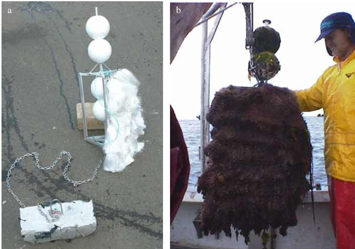
Plate 4.1 – Puerulus collectors a) design with two panels missing to show internal construction and, b) retrieved from site before being “banged”
