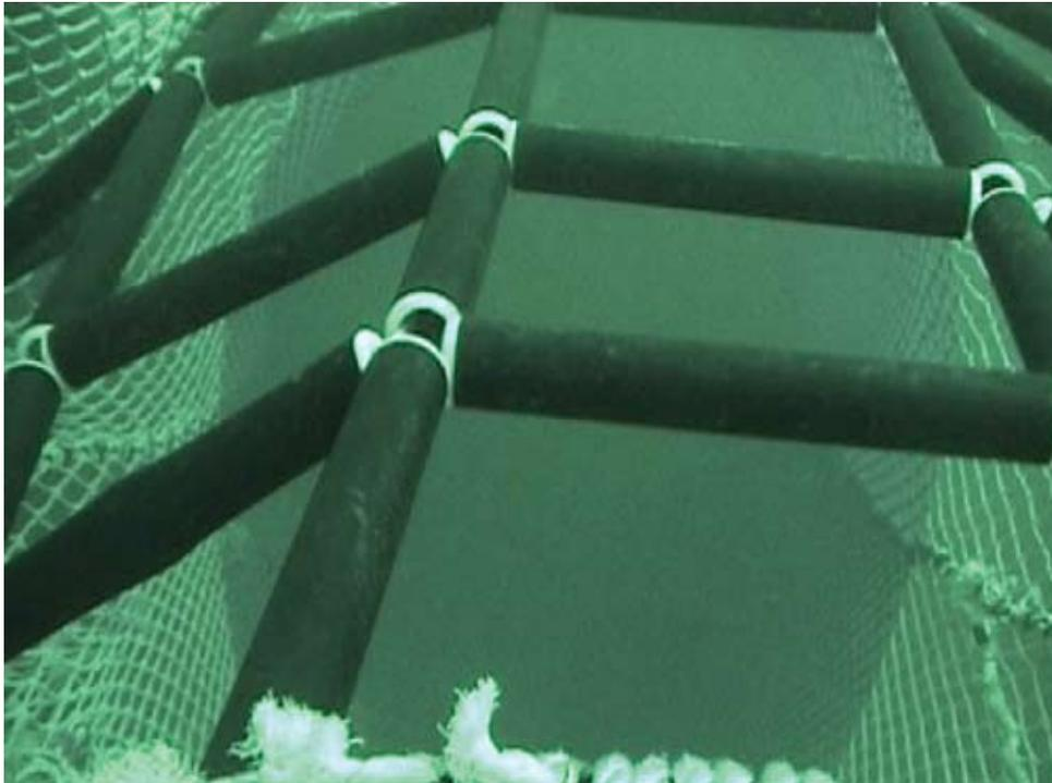
**Figure 15.** Flexible grid from Shetland, Scotland, with the camera downstream of the grid facing upstream towards the mouth of the net. The bottom of the grid, bound in rope, is elevated as the water flow is out the escape opening rather than through the grid.
