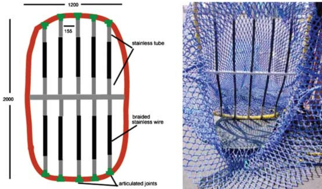
**Figure 13.** Semi-flexible grid constructed from stainless tube and braided stainless wire.
