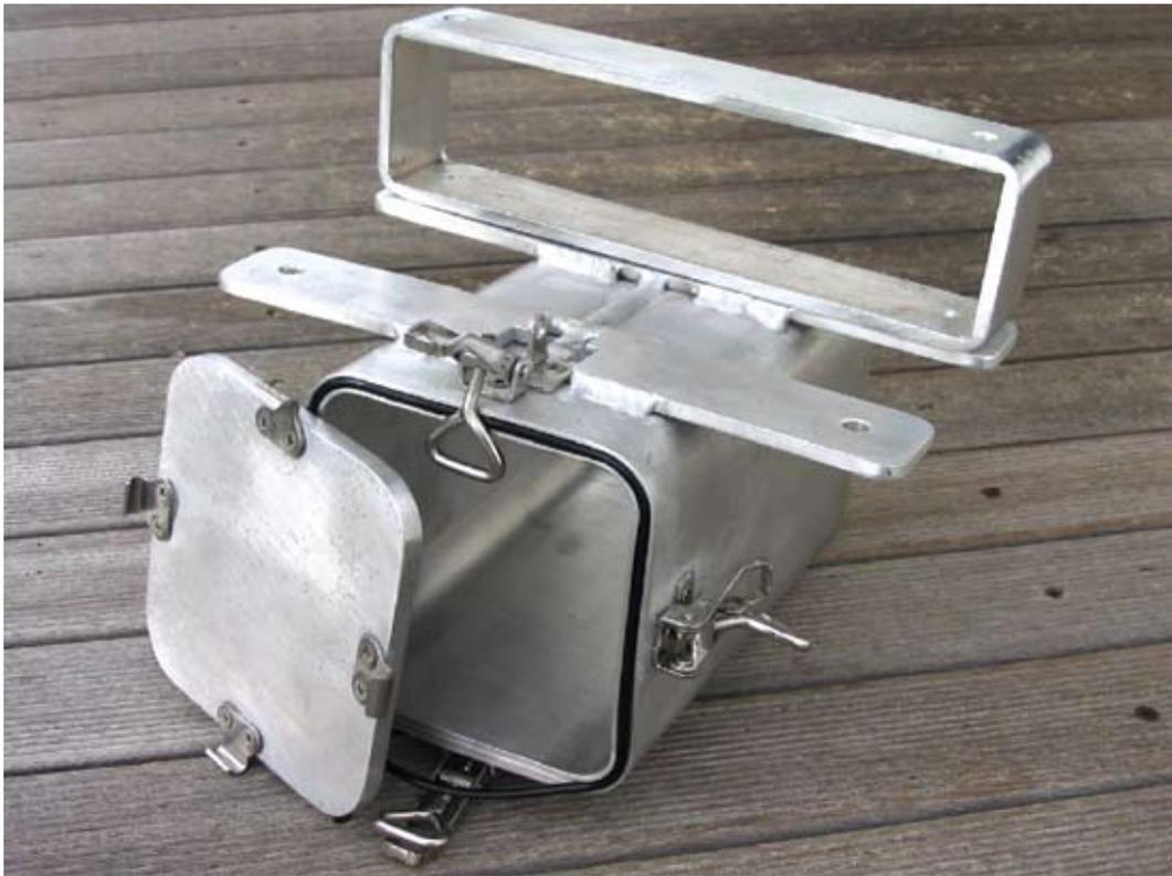
**Figure 11.** Under water video camera housing.
