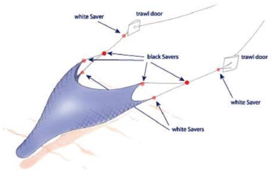
**Figure 12.** Positions of the pingers on the trawl net as suggested by manufacturer.
