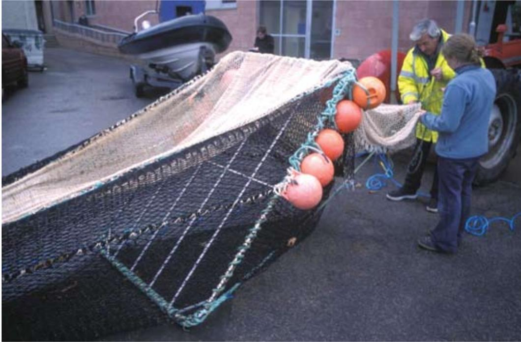
**Figure 5.** Solid metal selection grid used in trials in the UK sea bass pair trawl fishery between 2002 and 2004.
