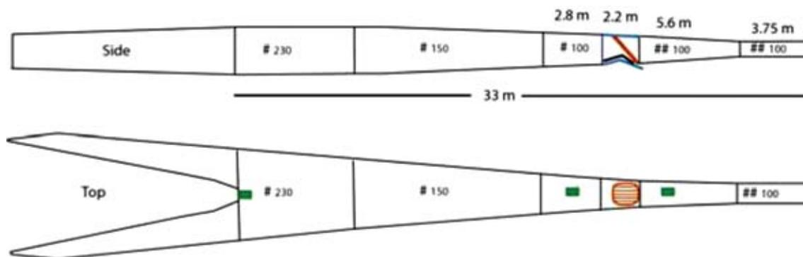
**Figure 14.** The plan of the net used during the trials of the selection grid showing the grid (brown), opening net cover (blue), Kevlar flap (black), location of the cameras (green) as well as the mesh sizes for the different panels of the net.
