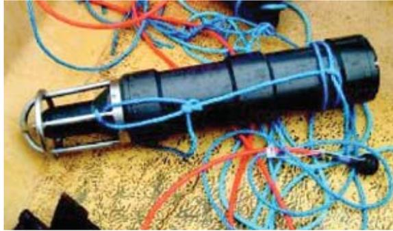
**Figure 4.** Aquatech pinger designed for the Irish pair trawl fishery and the area of deployment at the shark-teeth position in the net.
