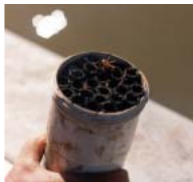
Figure 65. A) Purse type puerulus collector so different sizes. B) PVC tubes inserted into purse collectors.
