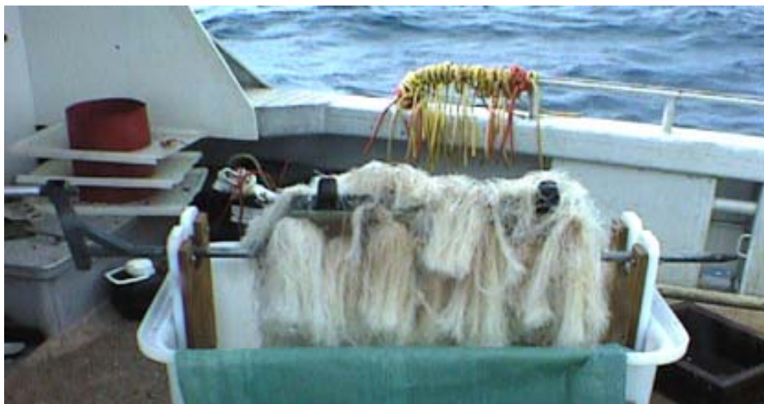
Figure 4. Spinning tub for sampling collectors.
