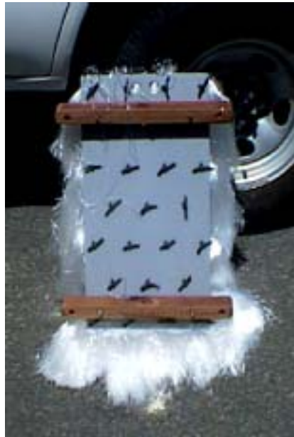
Figure 2. Internal side of the sandwich collector.
