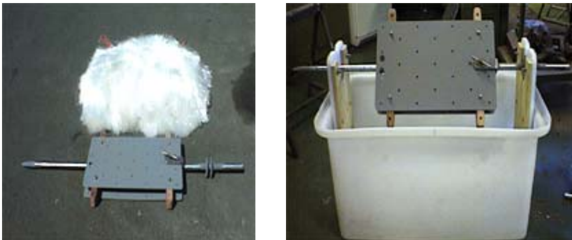
Figure 3. Location of spinning shaft and spinning tub and holding brackets.
