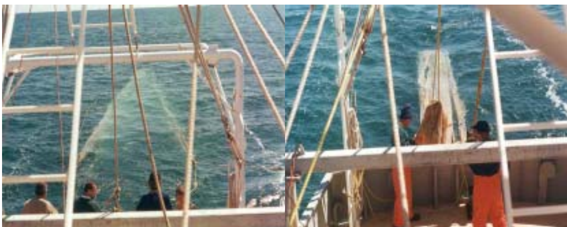
Figure 75. (left) Mid-water trawl net being trialled off Fremantle using R.V. "Flinders". (right) Net being shot away and net being retrieved.
