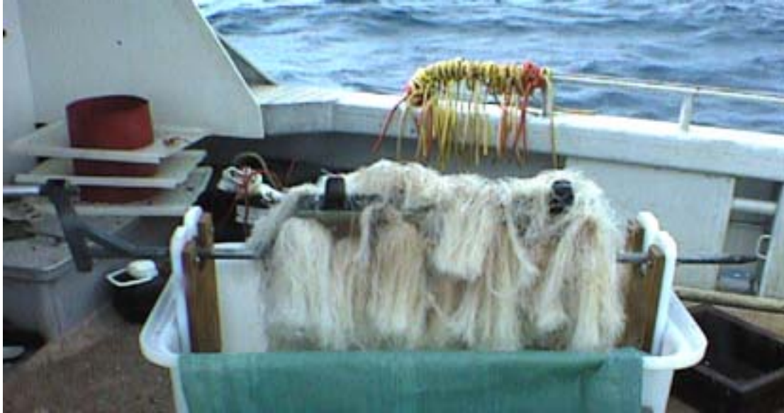
Figure 62. Spinning tub for sampling collectors.
