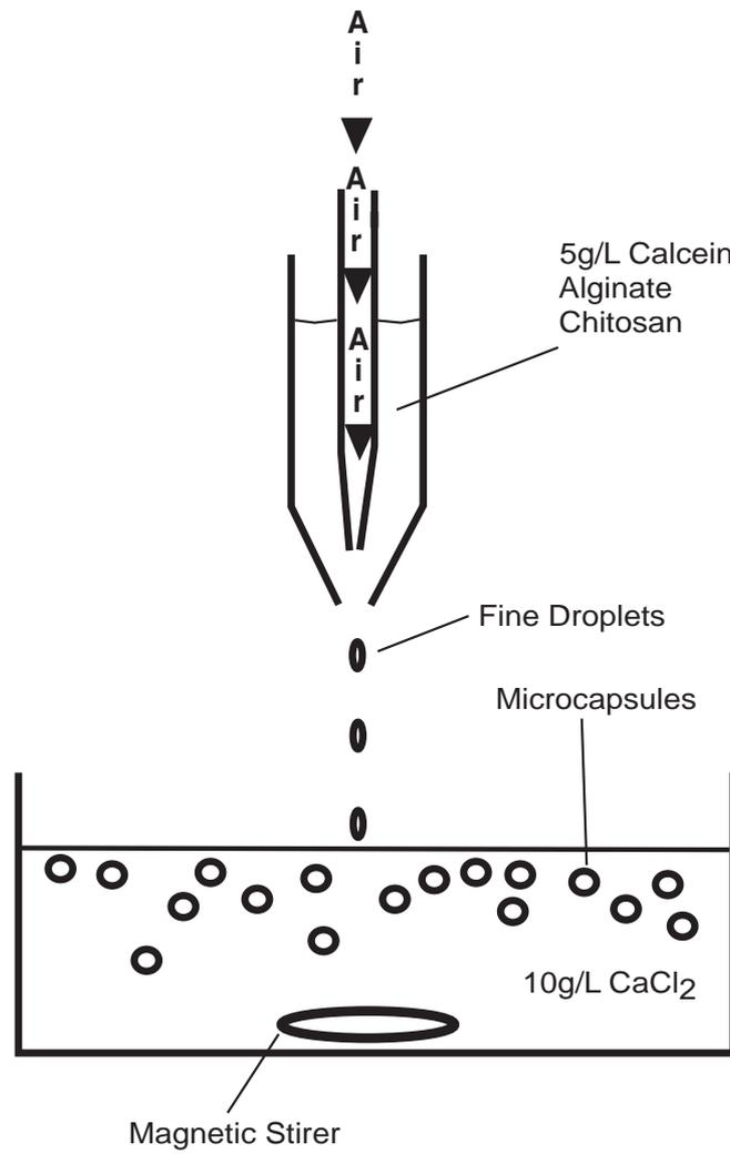
**Figure 6.** Shows the procedure and apparatus used in the preparation of calcein microcapsules that were mixed with food and fed to a number of *Sardinops sagax* held in a sea cage.
