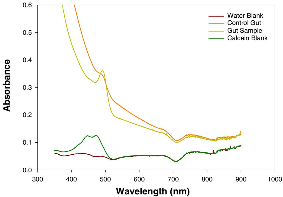
**Figure 23.** Spectrophotometric analysis of gut samples taken from *Sardinops sagax* to determine if calcein is active in the stomach after they were given calcein microcapsules in their food.
