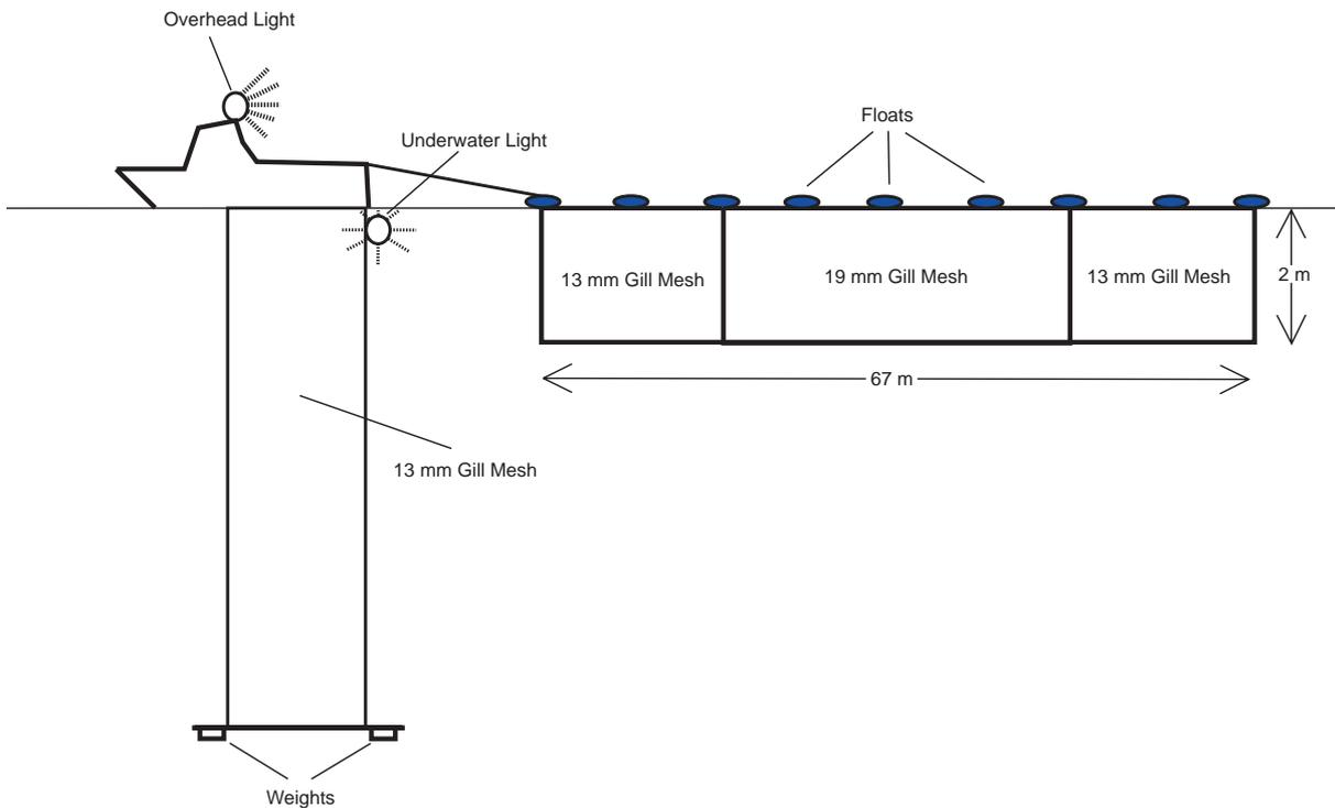
**Figure 3.** Diagram showing how the two types of gill nets were deployed for the capture juvenile *Sardinops sagax*; a 67 m long floating gill net with a 2 m drop, and a vertical gill net hanging from the gunwale of the vessel to the ocean floor.
