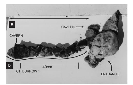
Figure 4. Polyurethane cast of a yabby burrow displaying measurements of depth into dam wall (a) and actual burrow length (b).
