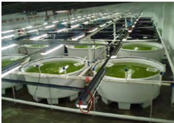
Figure 2. Photograph of the GFB Fisheries Ltd hatchery showing typical tank design and operation of a greenwater culture.
