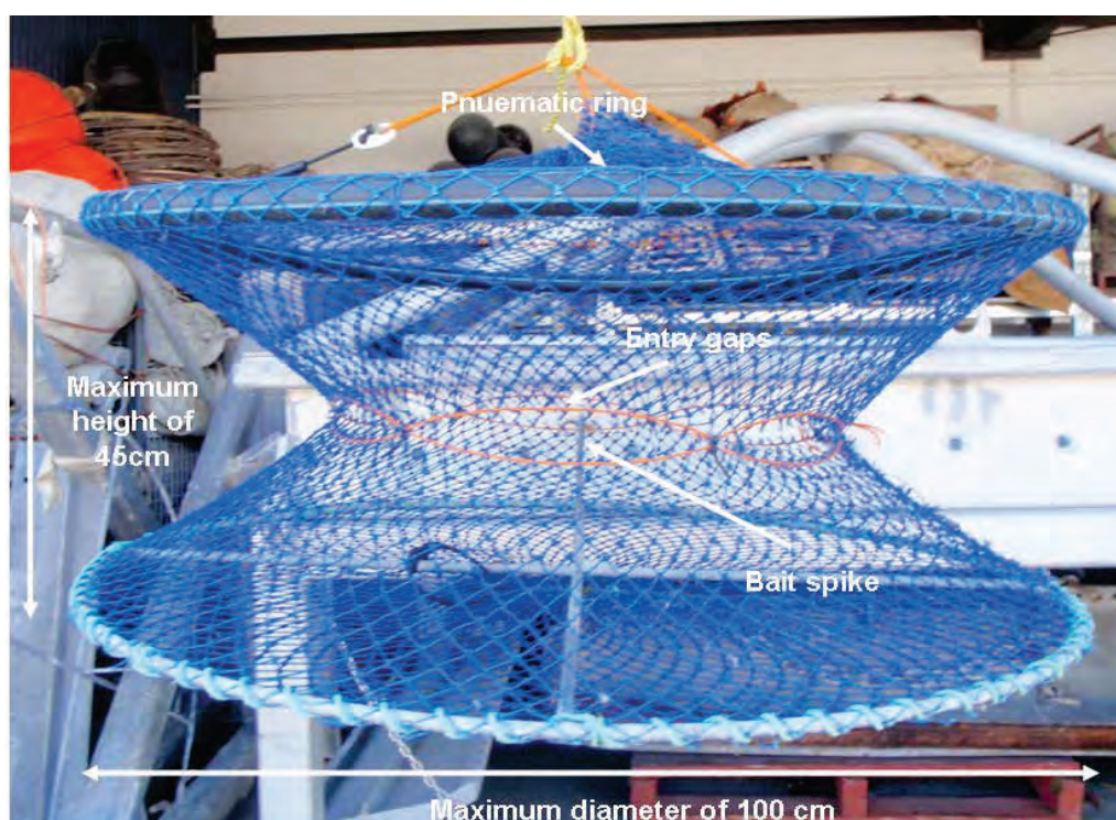
Figure 8.4. Hourglass research crab trap used in the fishery-independent monitoring surveys in the PHE (Photo credit: Chris Marsh [DoF]).
