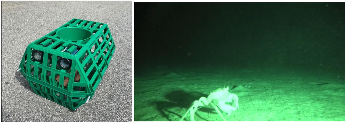
Figure 5-17 Images of (left) commercial WCDSMF crystal crab pot fitted with light and camera system, and (right) crystal crab and associated habitat.
