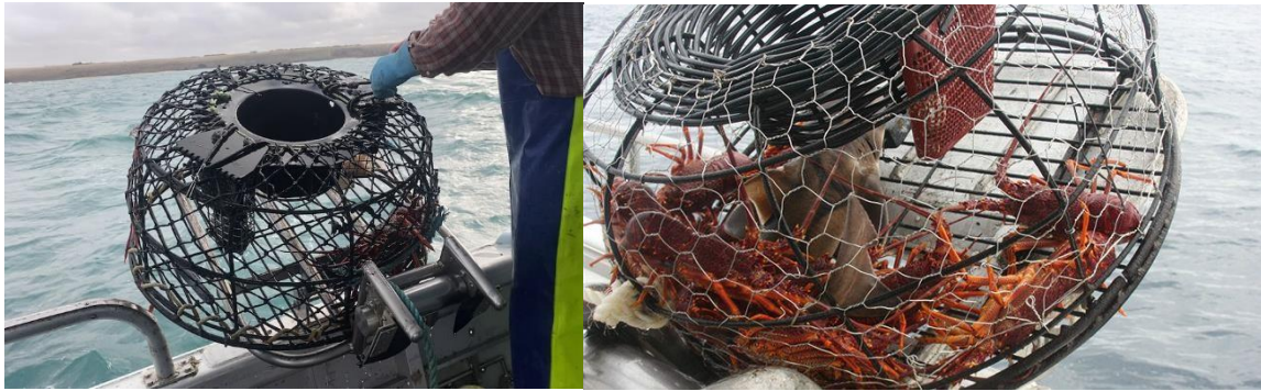
Figure 4-9 Two examples of steel frame “beehive” pots covered with trawl mesh (left 1 ) and chicken wire (right 2 ).
