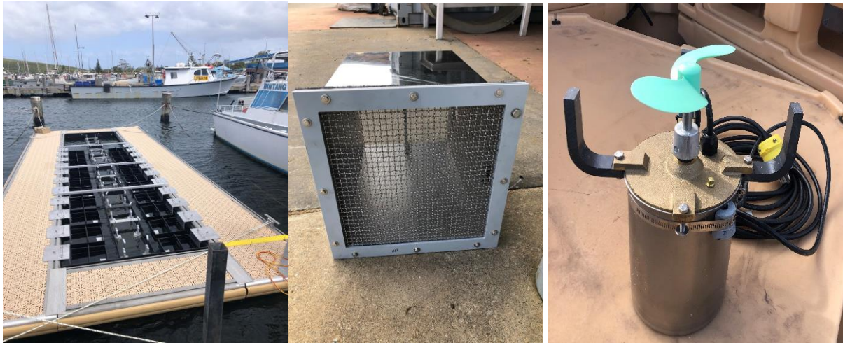
2 Left- Completed FLUPSY at "C" jetty. Middle- FLUPSY pot showing the screen bottom. Right- Spare pump.
