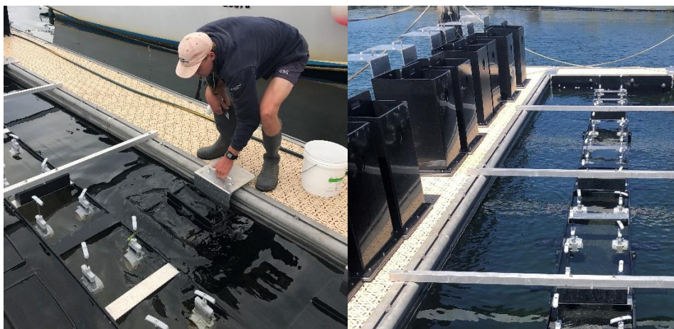
9 Left- Lifting upwellers from the water. Right- upwellers sitting on the FLUPSY deck.
