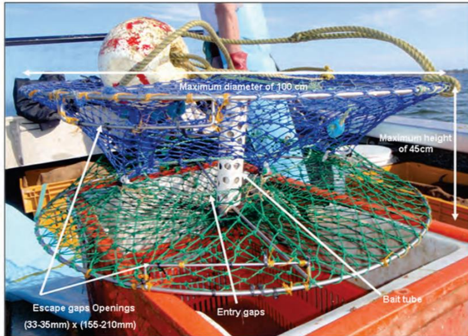
Figure 5.2. Commercial crab trap used in the Peel-Harvey Estuary, showing escape gap at the bottom. Source: Johnston et al. 2015.
