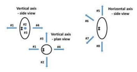
Figure 6 Schematic showing alarm measurement orientations, 4 from the vertical axis (at 90° angles) and 4 from longitudinal axis (at 45° angles)
