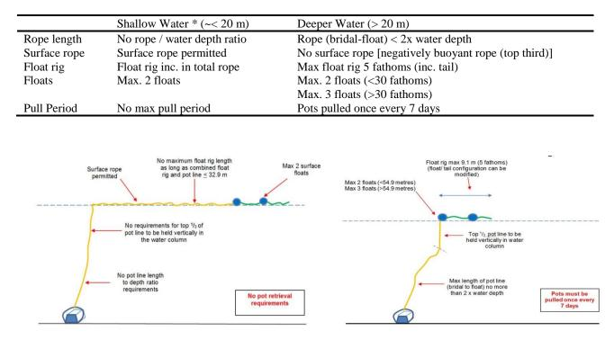
Figure 2 Diagrammatic representation of the gear modifications required in a) shallow ( $\sim$ <20 m) and b) deep ( $\sim$ >20 m) water depth
