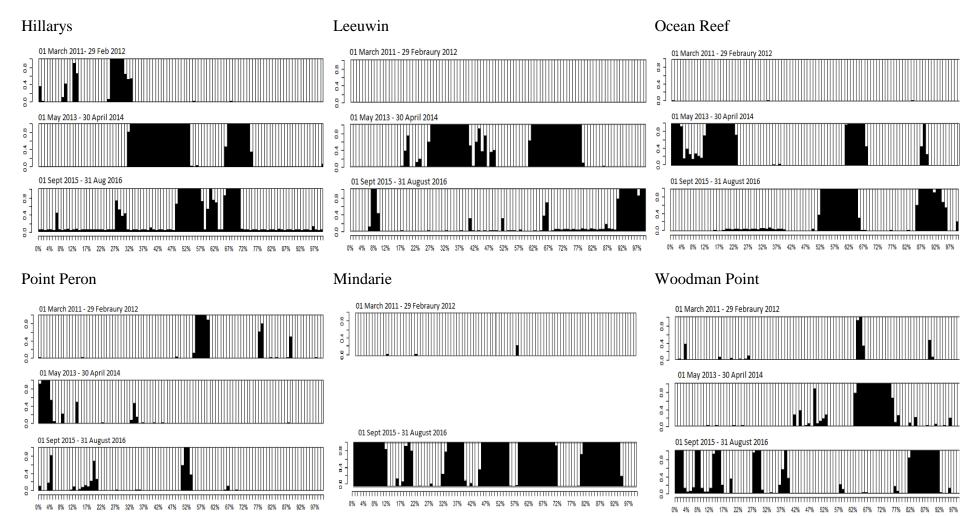
Figure 2: Distribution of the outage patterns. The black shades represent duration of outages and the white shades represent duration of no outages. The horizontal axes represent the percentage partition of the length of the data points (8784 hours for leap year and 8760 hours for non-leap year). The vertical axes represent the percentage of missing data in the percentage partition of the data points.
