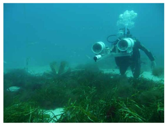
**Figure 2.1** Image of sDOV in use illustrating size, position of synchronising diode and positioning of inwardly converging cameras in housings.
