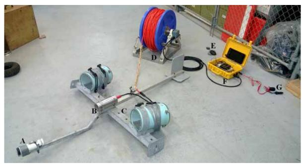
**Figure 2.2** Towed underwater video setup utilised on the smaller research boat where Asynchronisong diode, B- live feed video camera, C- BRUV crossbar with stereo video housings, D- live feed video cable, E- GPS overlay antennae, F- topside case with monitor, video out plug and GPS overlay and G- 12v power supply .
