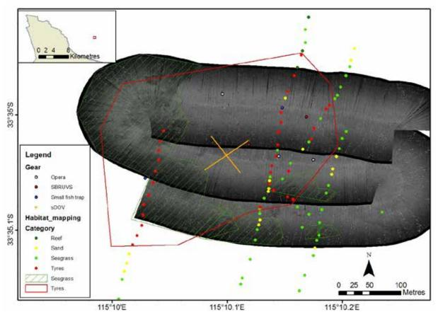
**Figure 7.12** Sidescan sonar map of Quindalup tyre artificial reef site showing sampling locations, towed video benthic habitat observations and indicating areas of seagrass (green hatching) and area with tyres (red).
