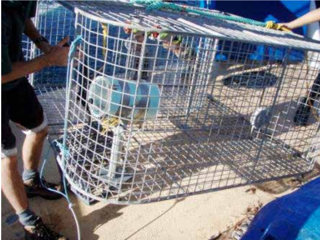
Plate 1. Example of video cameras in underwater housings mounted inside a fish trap.
