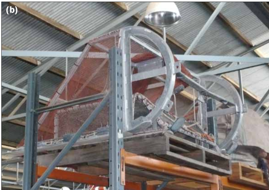
Figure 1. a) Early prototype benthic dredge employed by SARDI. b) Later prototype dredge employed by SARDI.
