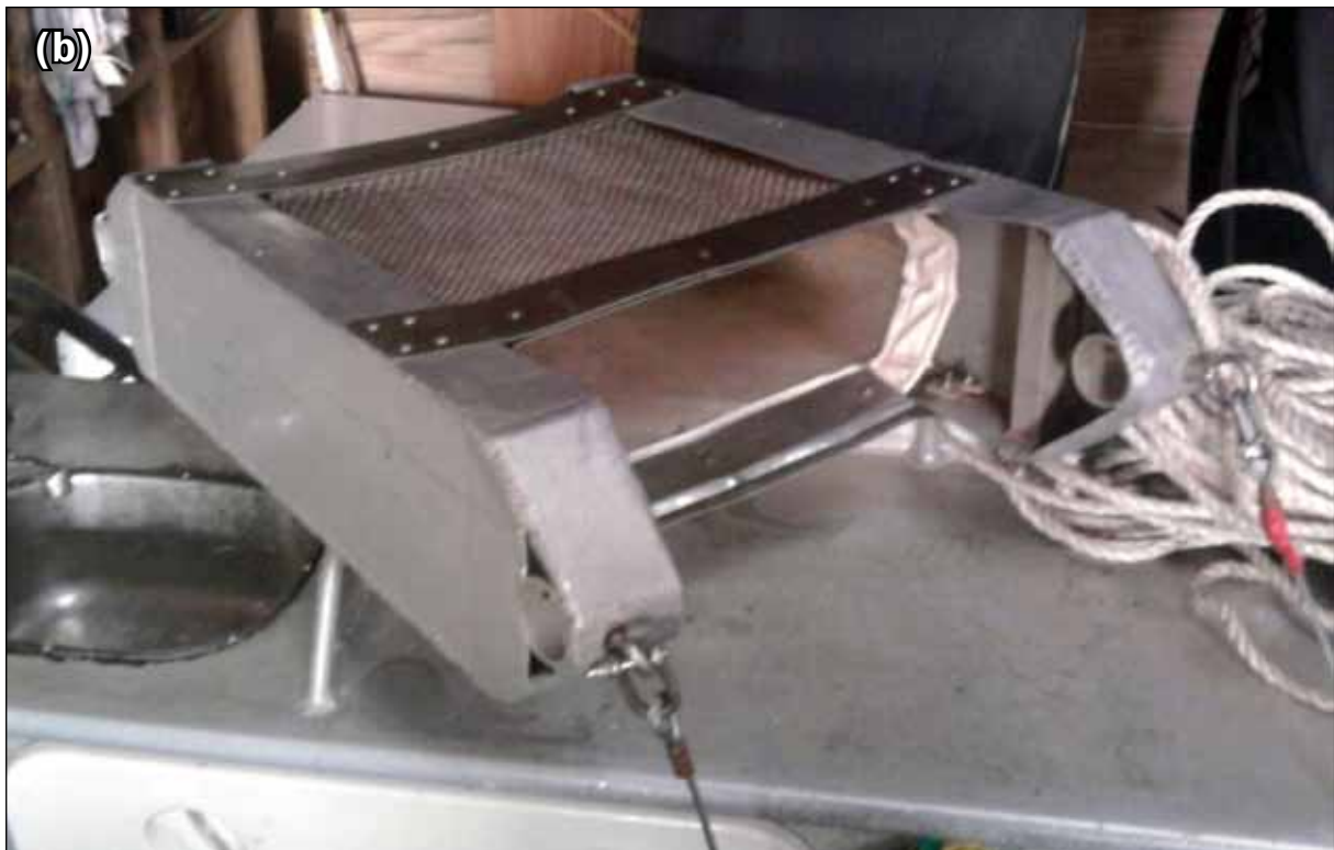
Figure 2. a) Large Ockelmann sled employed at SARDI. b) Small Ockelmann sled employed by NIWA.
